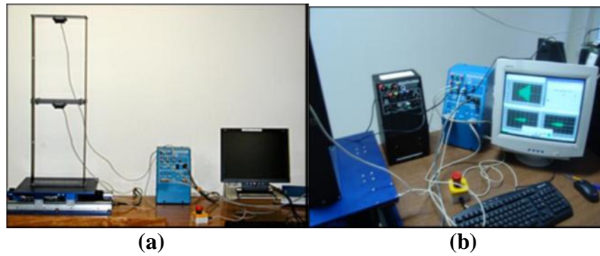
Figure 2a, b Illustration of model steel structure and shake table
